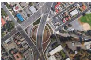
**Median.** Median island reconstruction to support 2-way movements in and around Foothill Blvd/Mission Blvd/D St. intersection
