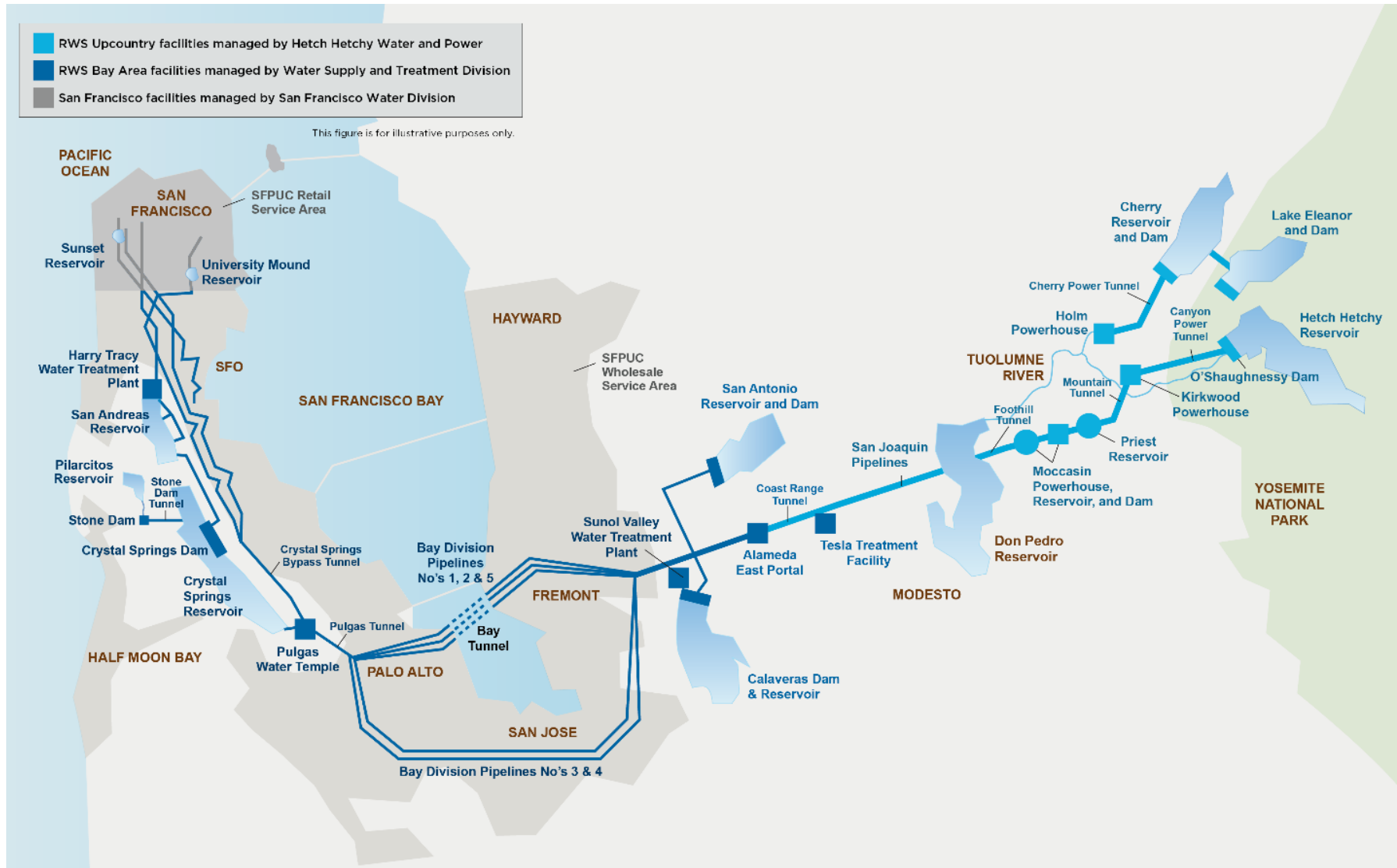
Figure 6-1. SFPUC's Regional Water System and Main Facilities
