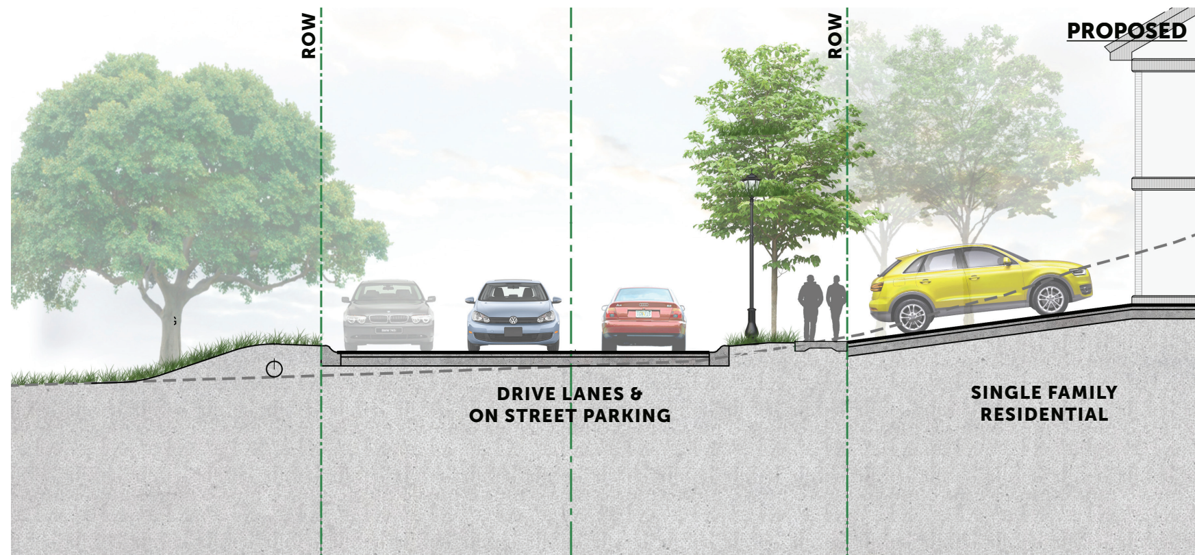
Figure 4-8: Maitland Drive Proposed Development Typical Street Section
